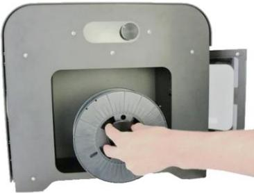
Press the button on the status screen, select Spooling in the Main menu > Start Spooling and follow the steps shown on the display of the filament maker. When the set diameter is reached, cut filament below puller. While guiding the filament through the filament maker following the screen instructions, fasten the filament on the spool.
