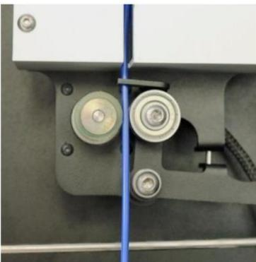
Let it run for a couple minutes until it works properly. The filament is ready to be wound on the spool when the measured value of the optical sensor is the same as the set value.
